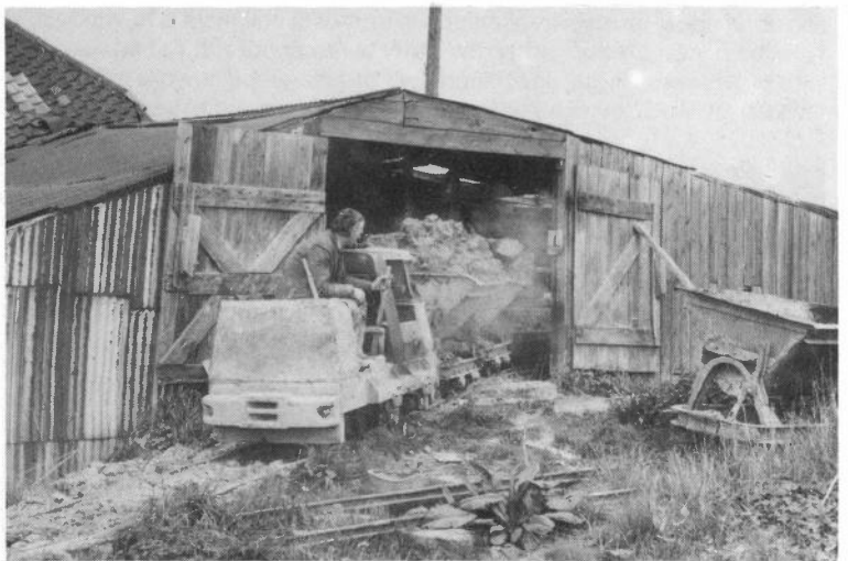
Ruston & Hornsby 247182 struggles up the final incline into the tipping shed, with a load of freshly excavated clay. (A.J. Booth)
