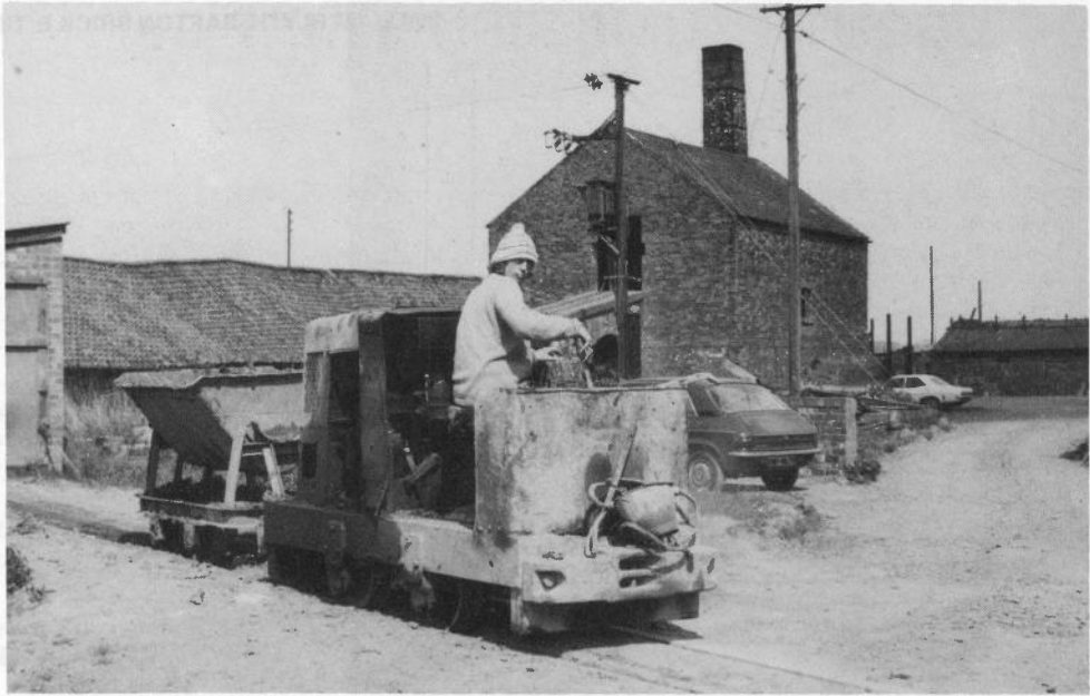
Ruston & Hornsby 260708 sets out from William Blyth's Far Ings Works for the clay pit. The loco shed is just visible on the extreme left of the photograph. (A.J. Booth)
