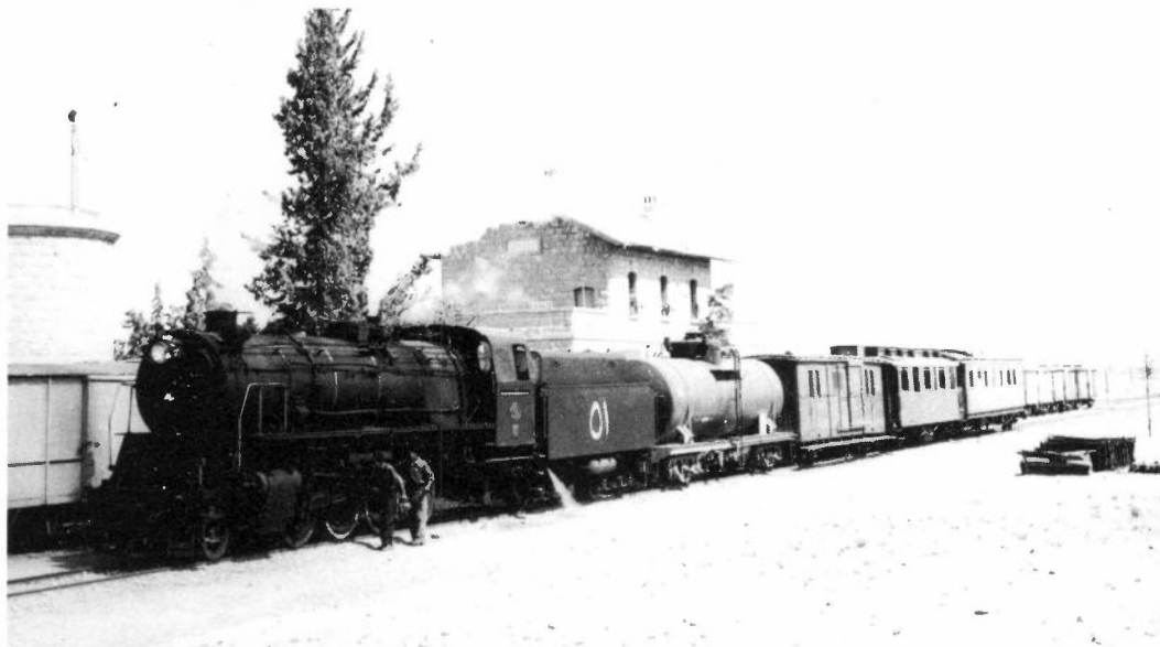
Our special train from Amman to Quatrana makes a refreshment stop at Khan Zibib. The loco crew take the opportunity to oil round Jung 2-8-2 No 51. (K Taylorson)
