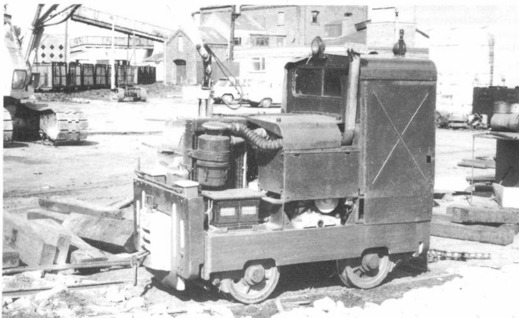
The 48 hp Motor Rail locomotive, works number 40s378, at Hatfield on 9th April 1977. (A.J. Booth)
