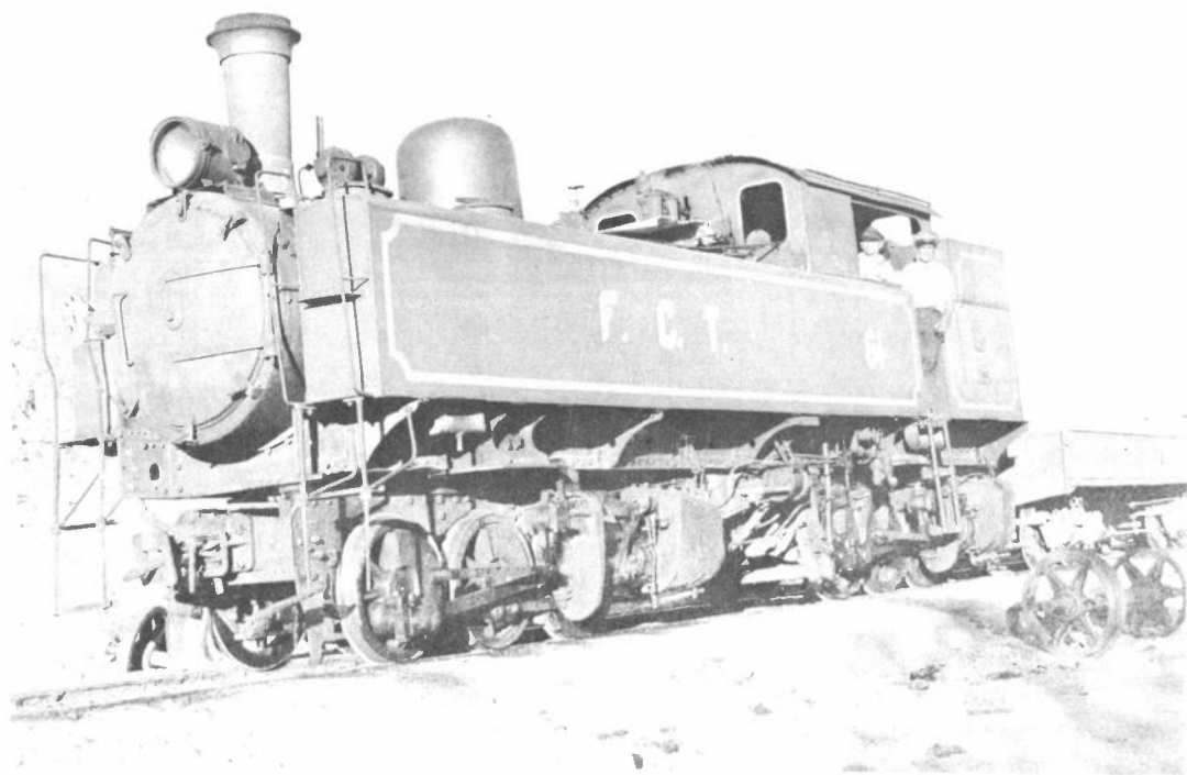
FERROCARRIL de TALTAL a BLANCA ESTELA (Gauge 3ft 6in.) No.61 0-6-0+0-6-0T Meyer by Kitson; at Taltal, N. Chile. (Dr. Roy Christian)
