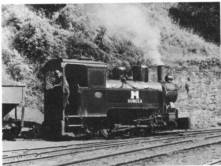
TURON COLLIERY, 600mm gauge No.16 0-6-0T, built Altos Hornos de Vizcaya in 1942, shunting the sidings September 1970. (Resplendent in lined green livery and displaying 'HUNOSA group' insignia.) (D. H. Wilson)
