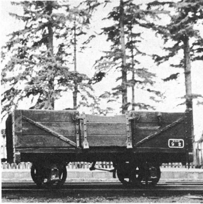
BELFAST & NORTHERN COUNTIES RAILWAY No.932. A 3ft gauge 4 wheel wooden wagon (fully sprung and hand braked) saved from the burners by Member W. P. McCormick and currently in use on Lord O'Neill's Shanes Castle Railway at Antrim in N. Ireland. (NGI.60/22-23). (The Lord O'Neill)
