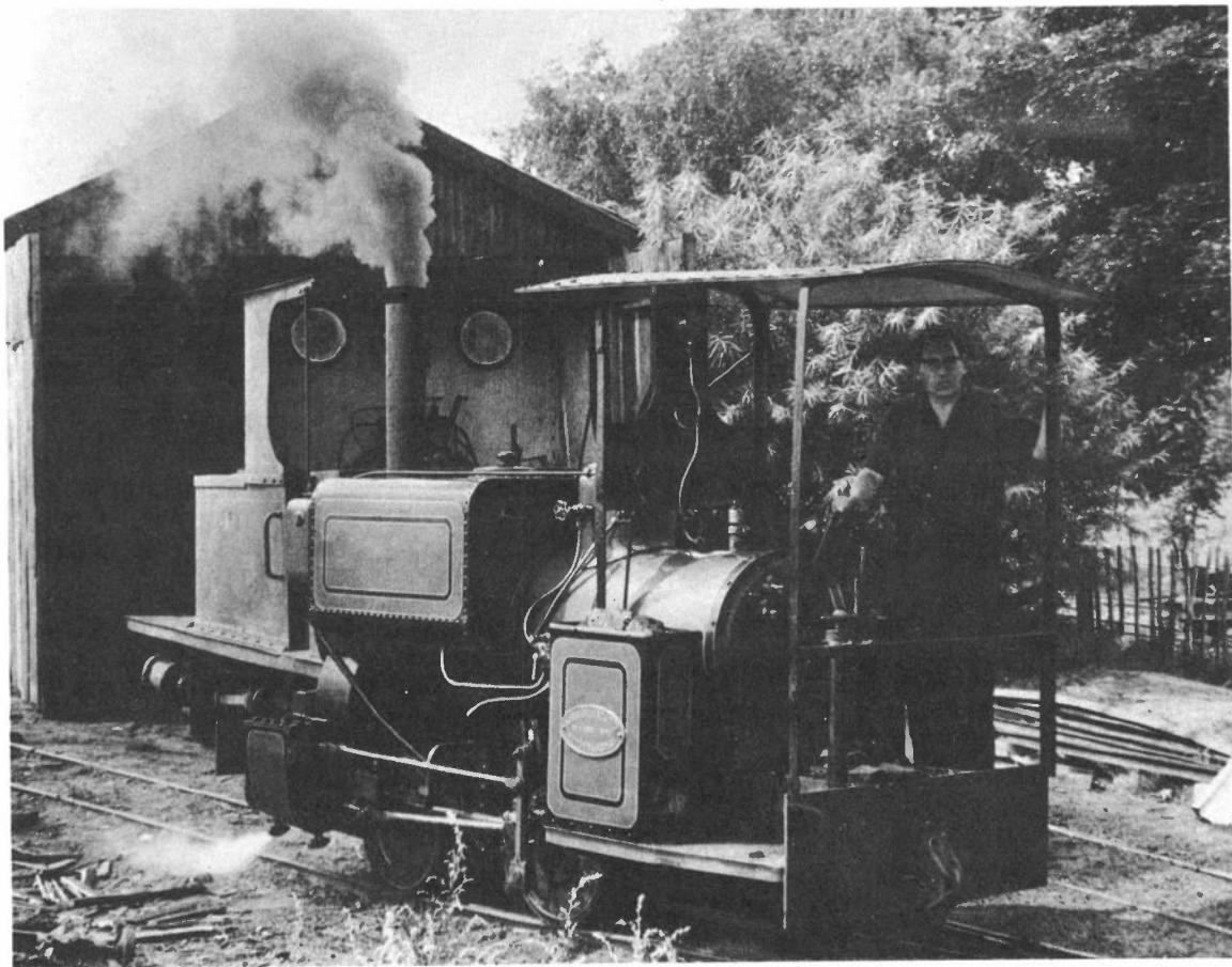
PIXIE (Kerr Stuart 4260, an 0-4-OST of 1922) steams away from Pages Park shed leaving THE DOLL (Barclay 1641) on an adjacent line.
