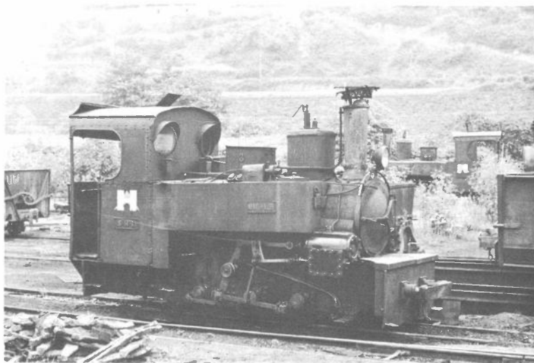
MINAS de ALLER. 600mm gauge. No.3 Corpet 467 of 1887, 0-6-0T (Note the motion!) vegetating at Ujo Depot, September 1970 (D. H. Wilson)
