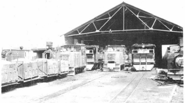
Outside Darnall Repair Sheds. The engines to the far left and far right are little Avonside 0-4-0Ts; the diesels are easy to spot, while the other visible steamers are Meyer Articulated. The front of the steam loco standing behind the central diesel can be seen . . . she was over what could be loosely termed 'the pits', and there was another Avonside 0-4-0T behind her.
