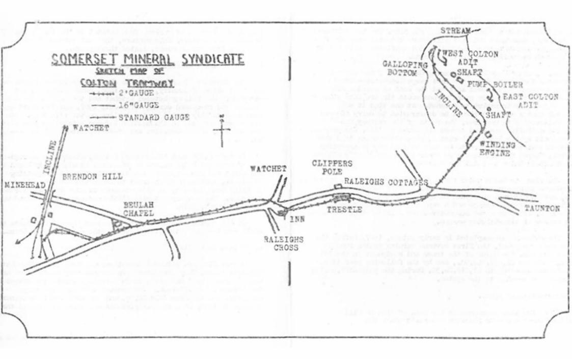
area they soon set to work re-opening the pits. The two entrances to the mine, East Adit and West Adit, were situated near the foot of adjacent valleys and a pump boiler and shaft were situated at the head of the valleys to serve the mine.
